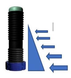
The lateral forces are based on the soil area that is calculated as the area of a triangle using ½ the base times the height. This is because the forces are greater at the bottom of thank and non-existent at the very top.
